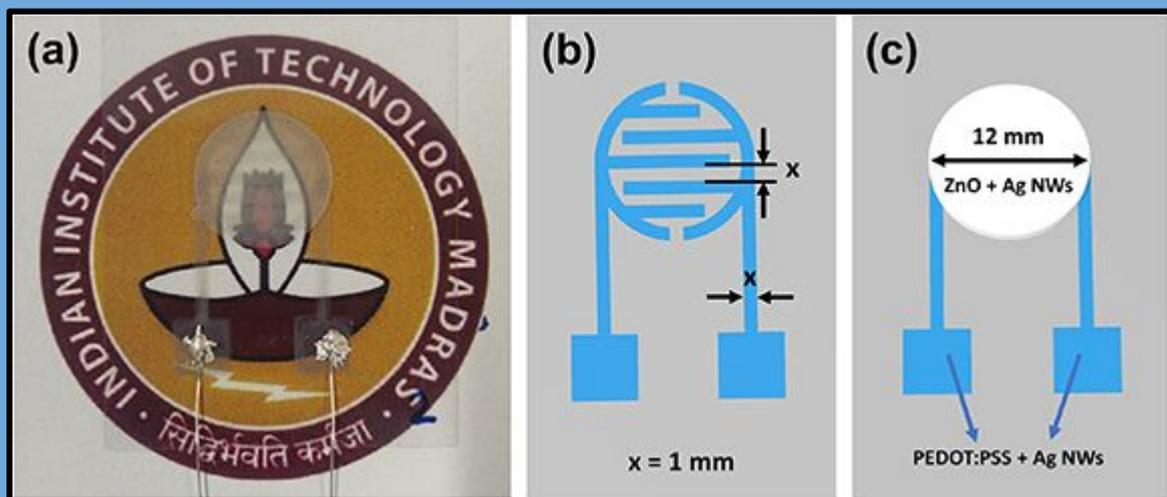
The structure of the fabricated PD. (a) The PD is placed over the logo of IIT Madras to demonstrate its transparency. (b) The dimensions of the printed electrodes and (c) the dimensions of the absorber layer and the materials used for the absorber and the electrodes.
