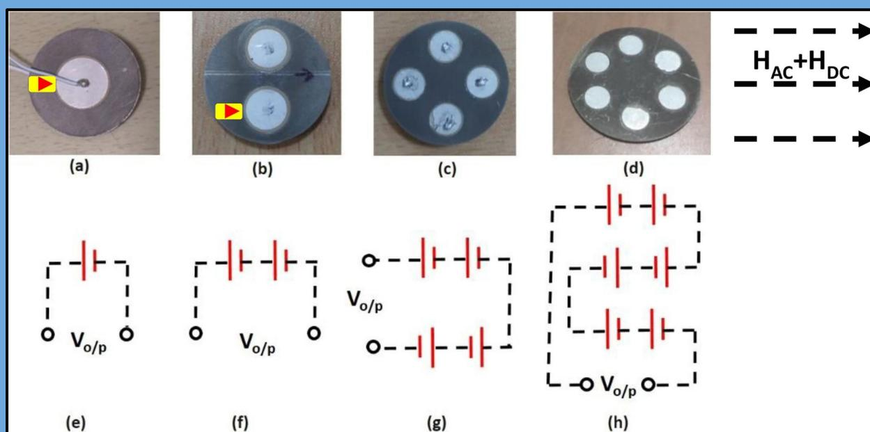
(a) Disc/Ring (b) DDS2 (c) DDS4 (d) DDS6 (e-h) Series connectivity of PZT discs in various configurations; (Note: grey-Nickel; white: PZT-5A; Yellow: Strain Gauge; Red Arrow: Direction of strain measurement).
