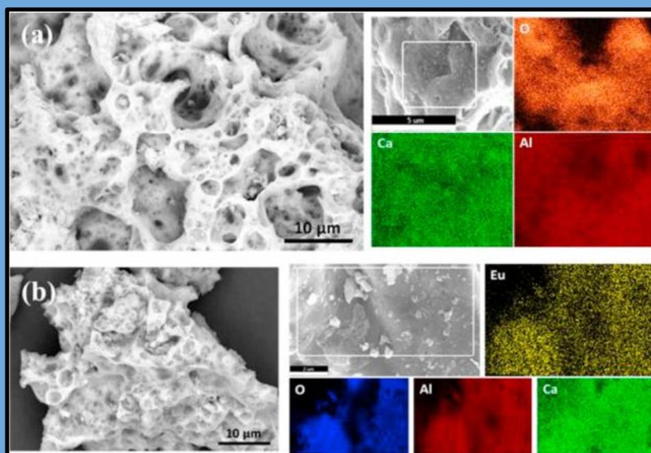
Scanning electron microstructures of the obtained porous Mayenite structures
