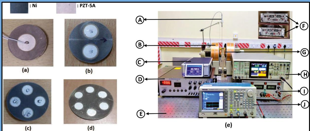
Fabricated configuration of ME composites (a) Disc/ring (b) DDS2 (c) DDS4 (d) DDS6; (e) Setup used for magnetostriction and ME measurement- A: Hall probe, B: Electromagnet, C: Gaussmeter, D: Strain indicator, E: Vibration isolation table, F: Power supplies, G: Helmholtz coil, H: Lock-in amplifier, I: AC amplifier; J: Function generator.
