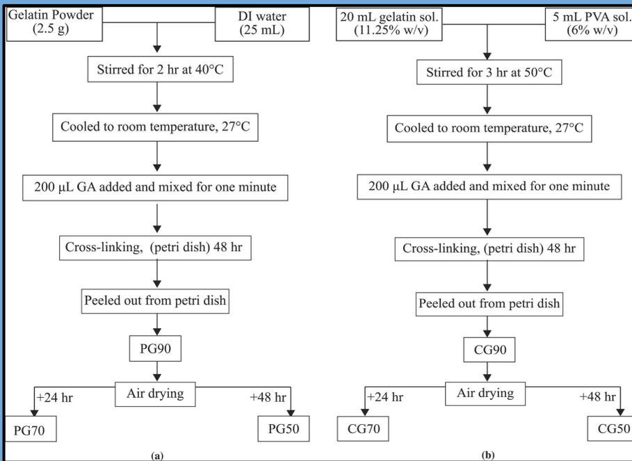
Schematic flowchart for the synthesis of (a) pure (PG90, PG70, PG50) and (b) composite (CG90, CG70, CG50) gelatin hydrogels having 90%, 70%, and 50% water content.
