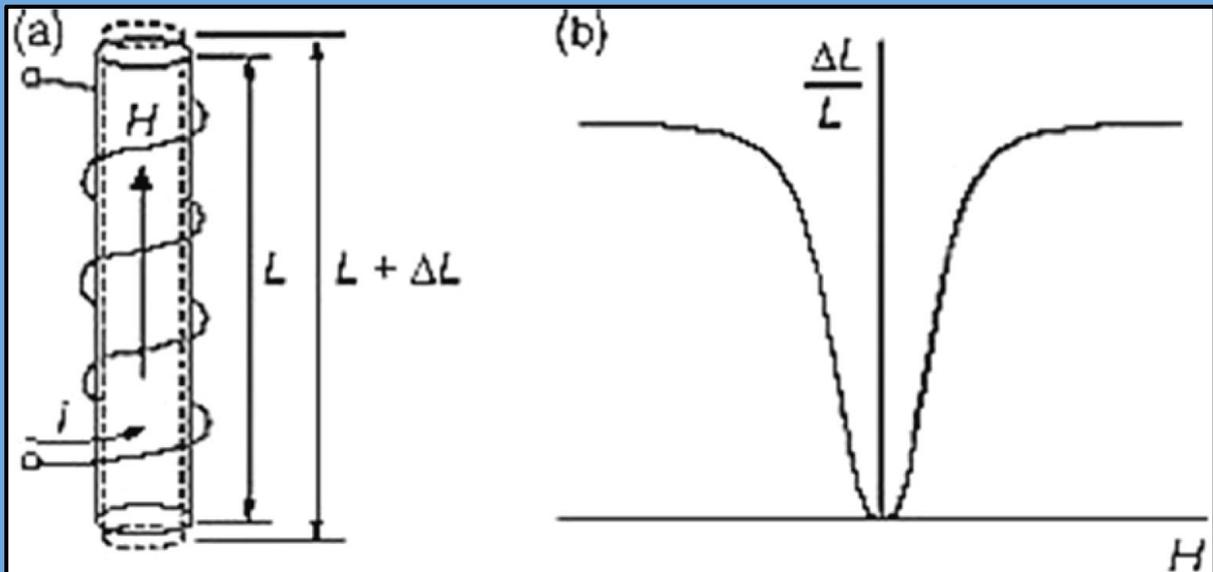
Schematic of the Joule magnetostriction observed in a magnetic rod (a) Change in shape with respect to applied magnetic field (b) Dependence of magnetostriction on
