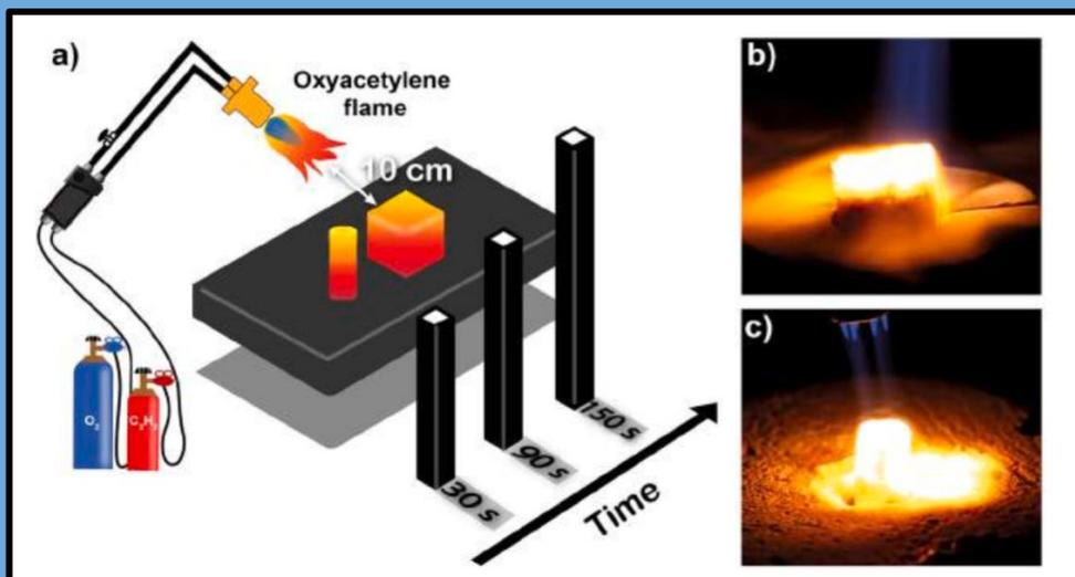
a) Schematic representation of the ablation resistance testing. Real-time photographical image of b) SiOC-OpenPF and c) SiOC-ClosedPF during ablation testing.
