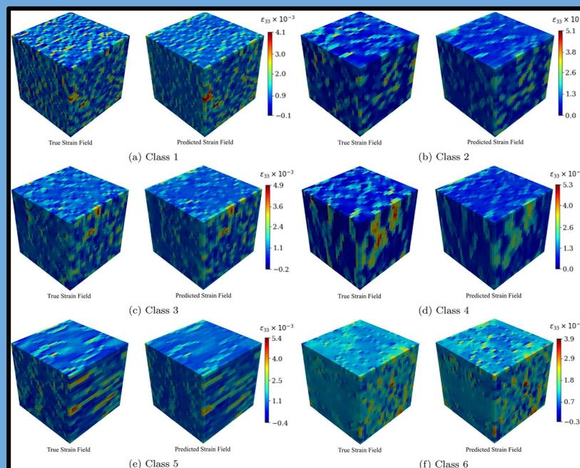
Comparison of the true strain field (from FEM) and predicted strain field (from UNet) on an arbitrary chosen RVE from each class (volume fraction 30%)
