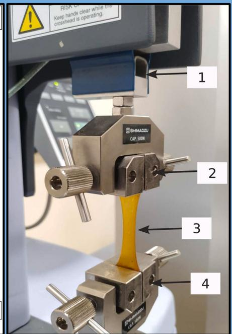
Experimental setup for the mechanical characterization using Universal Testing Machine, UTM
